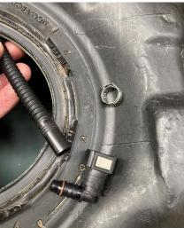
3) Fit the new right angle fitting to the internal fuel hose without tensioning the hose clamp.
