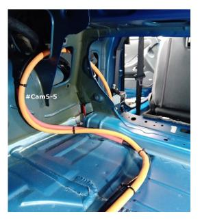
5) Single fuel module - connect the grey Anderson connectors.Dual Fuel modules - connect the grey and red Anderson connectors.
