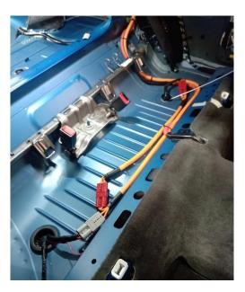
4) Continue to route the #Cam5-5 wire section towards the PWM Fuel controller in the spare wheel well.
