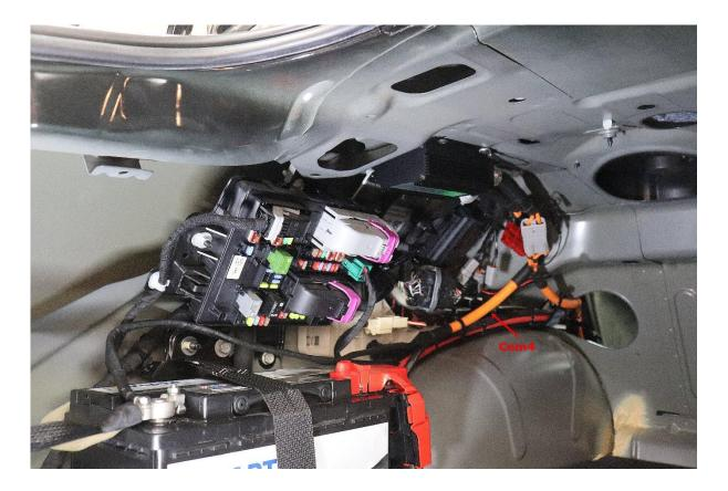
5) Neatly and securely fasten all cables as pictured with cable ties.
