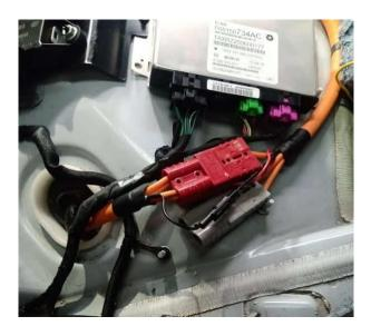
Finish the next section of wiring according the Primary Fuel Module installed in the vehicle.
