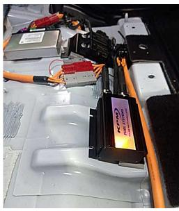
3) Be sure to mount the PWM controller small black earth wire/eyelet and screw down into one of the appropriate holes.
