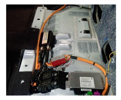
7) Route the #Th5 wiring loom to the large rubber grommet at the LH rear seat floor area to
