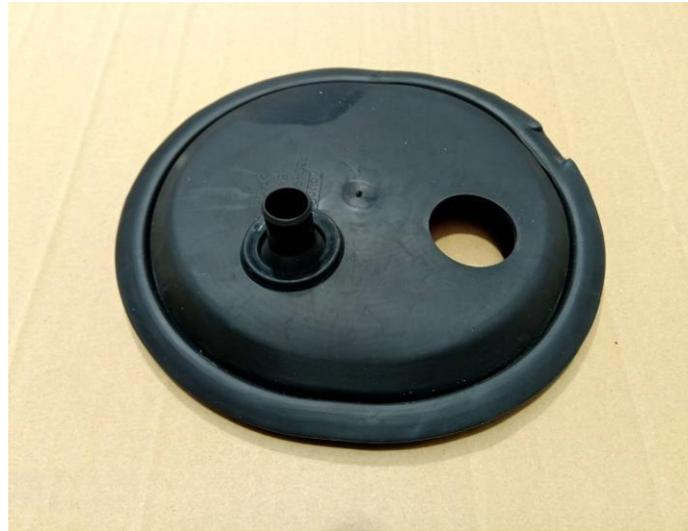
12) Remove the grey Anderson connector surround from the primary module cable (Mus5) and feed the cable through the new grommet.
