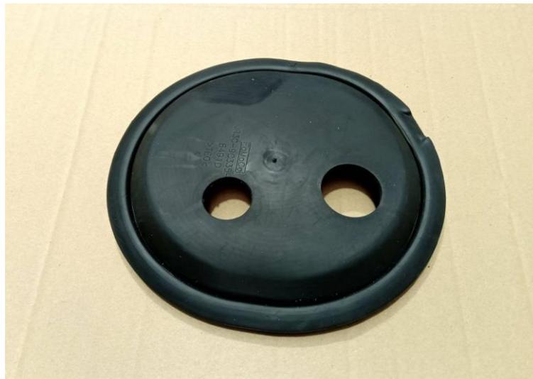
11) Fit the new supplied 30mm grommet as shown.
